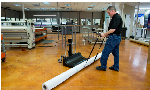
Safety straps pull rolls onto the tray with minimal effort.
