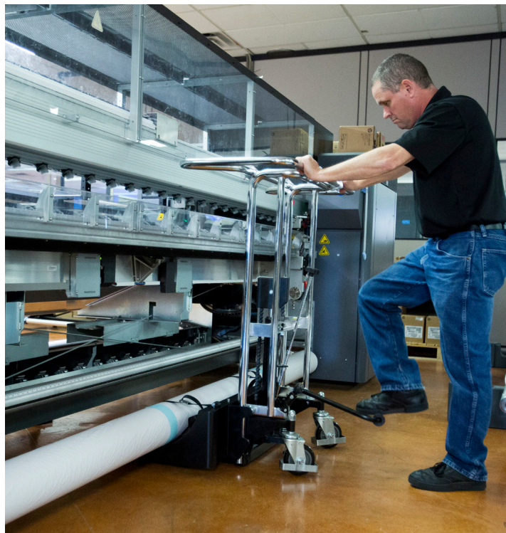
Specially designed low Profile tray and casters fit inside the printers roll loading area.
