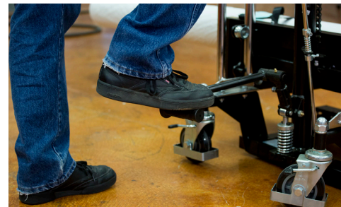
Easy to operate foot pump raises roll to correct height for transport and loading roll into the printer.
